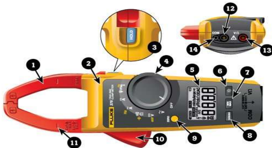
figure 2.27 clamp ammeter parts
