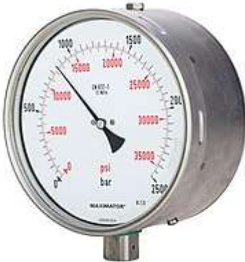
figure 2.28(a) Bourdon pressure gauge figure 2.28(b) reading psi (red scale) and kPa (black scale)
