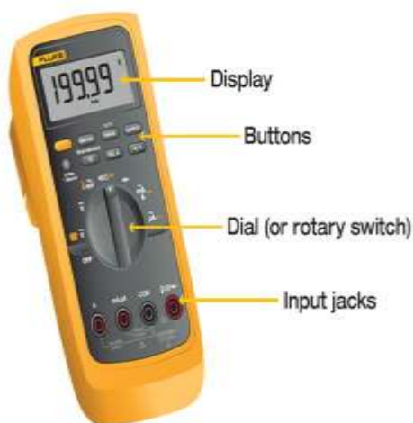
figure 2.24 components of multi meter
